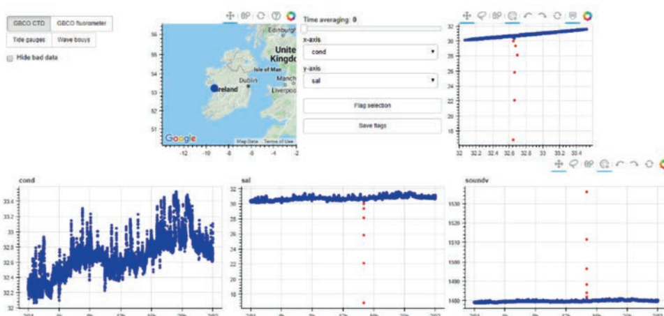
Fig. 2 - Example of data screening GUI implemented using interactive visualisation toolbox.
