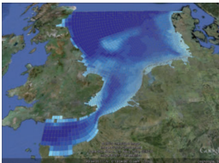
Fig. 2 - High-resolution output of Delwaq Model stored as netCDF.
