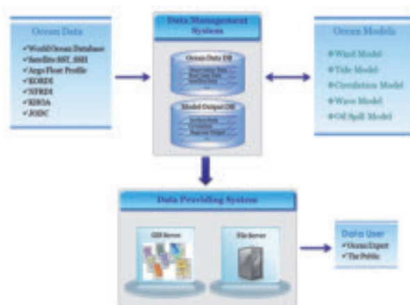
Fig. 1 - Structure of the operational data management systems for KOOS.
