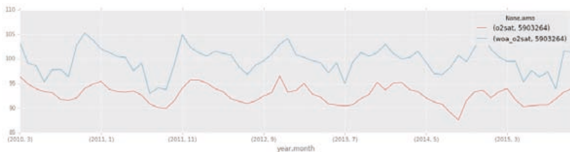
Fig. 2 - Over 5 years of surface oxygen saturation measured by Bio-Argo float 5903264 (blue) compared with oxygen saturation from the World Ocean Atlas (red). The biofloat Python software enabled easy generation of this plot in a Jupyter Notebook.
